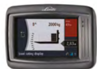
System wspomagania operatorów Linde Safety Pilot
